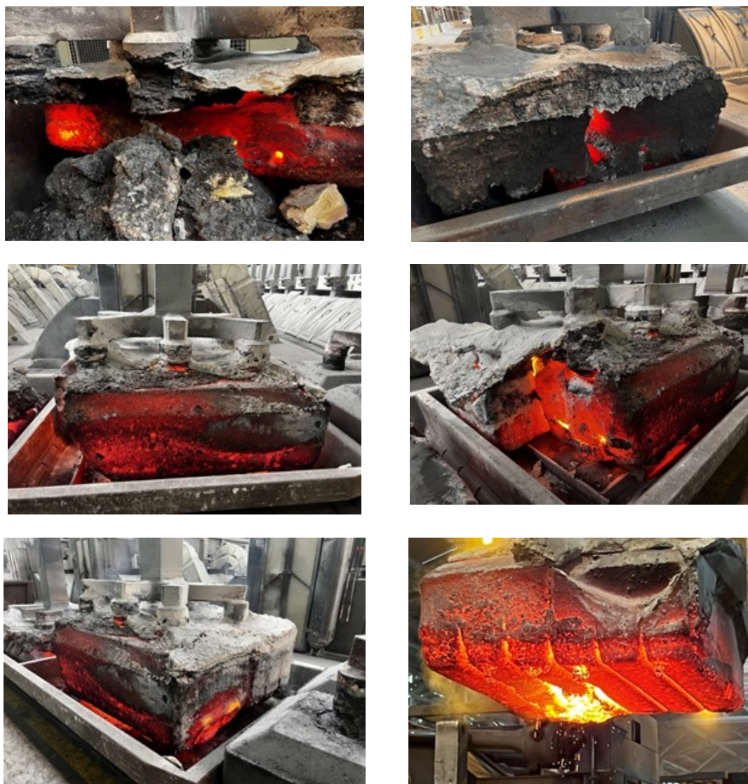
Figure 2. Type of anodic incidents and fallen blocks.
